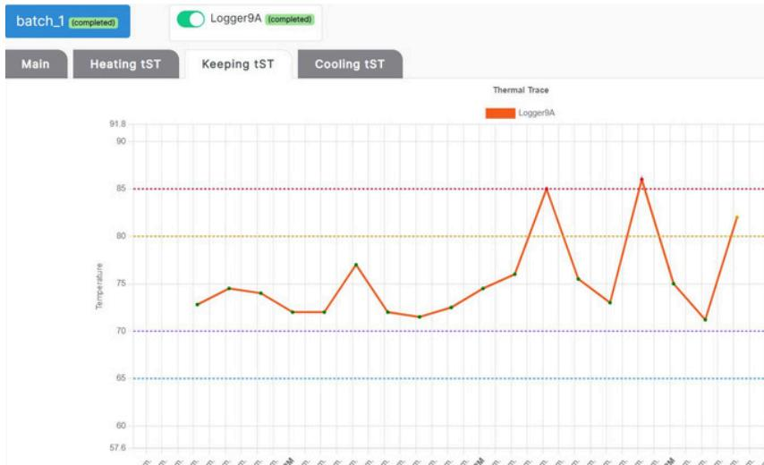
Operators can examine the cooking and cooling of a batch with a predictive curve that will warn the users if the recipe will complete at the appropriate temperatures at the scheduled time.
