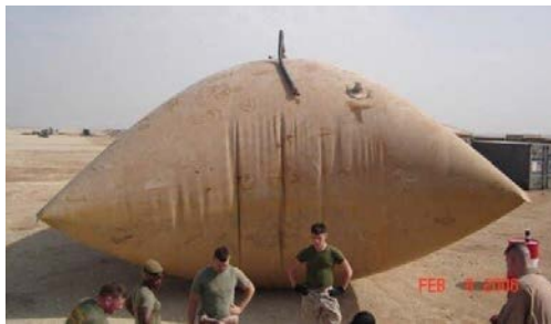
Air testing a huge fuel bladder for leaks before filling up with aviation fuel, critical for U.S. & Coalition aircraft operations.
