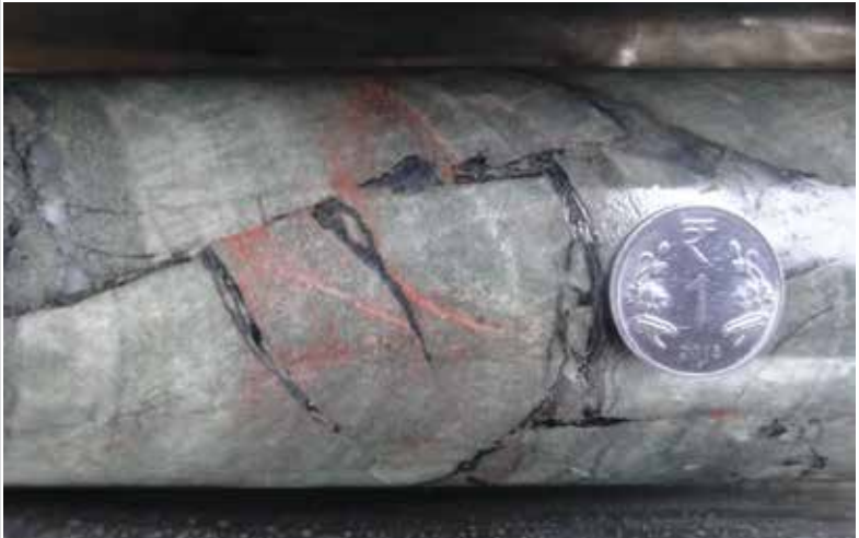
This core sample obtained from drilling shows master fault and pseudotachylite veins in the granite rock underlying Deccan basalt, providing direct evidence of earthquake activity (coin shown for scale)
