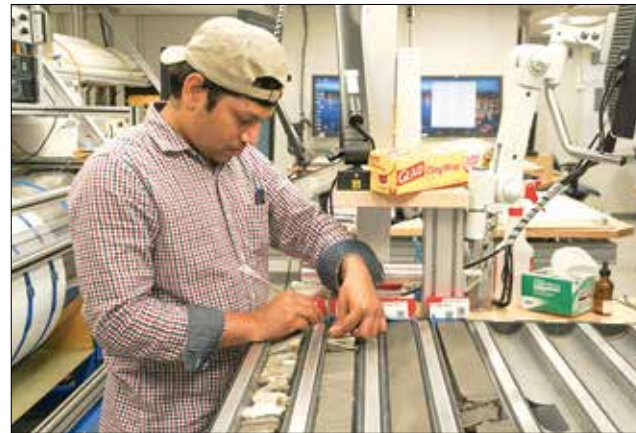
A sedimentologist takes a small amount of sediment from a core section to examine the microscopic constituents of the sediment
