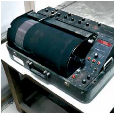
Analogue smoke paper type seismograph
