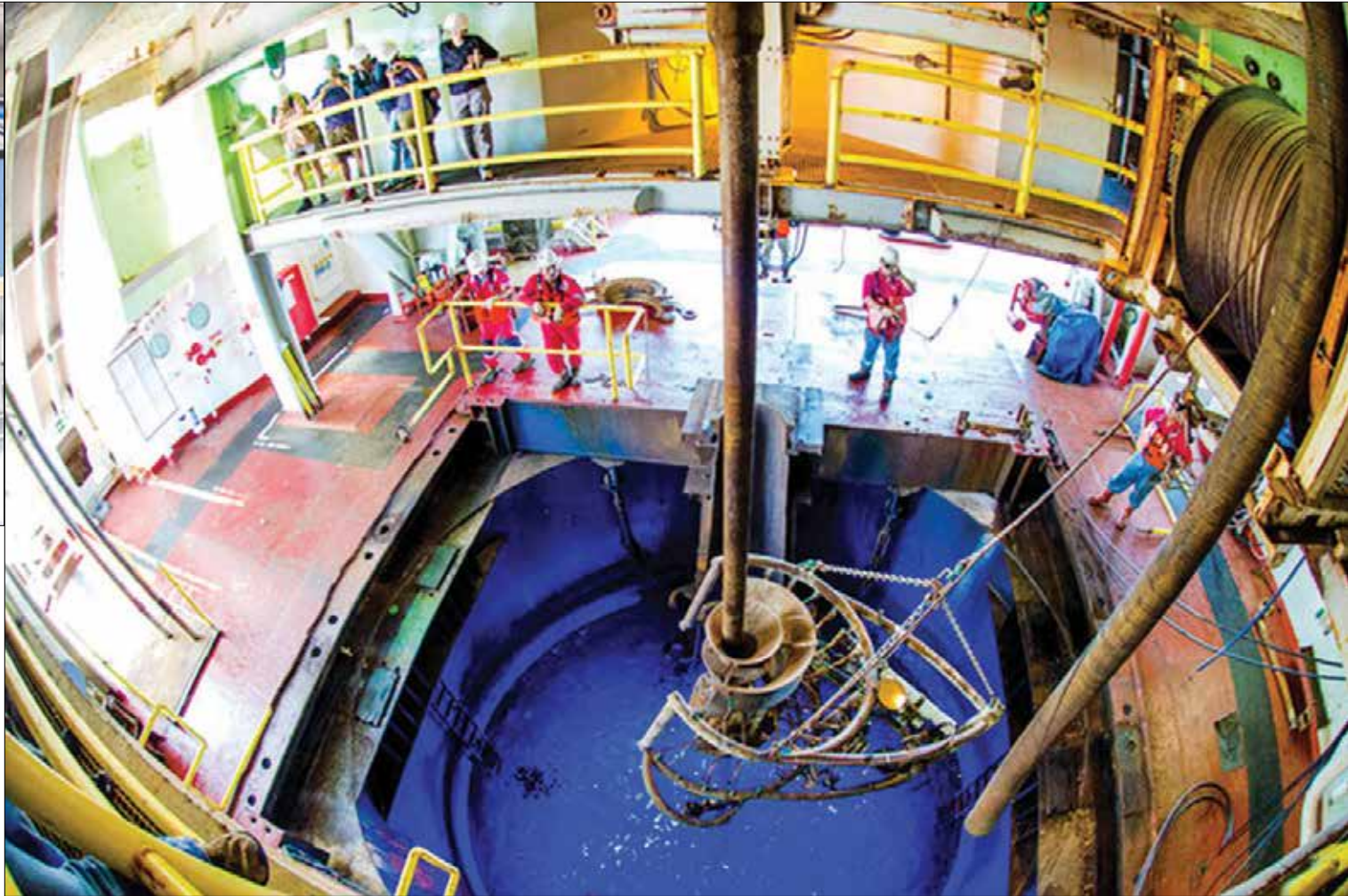
Subsea camera system being lowered into the cyan blue waters of the moonpool during Exp 355
