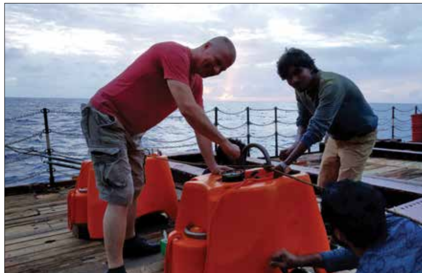
The scientific team assembling an OBS system on board ORV Sagar Kanya
