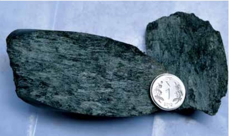
Core sample showing prominent slickenside with slickenlines observed on a fault surface (coin shown for scale)
