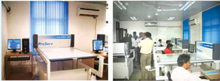
Instrumentation set-up for digitising analogue charts: » 5-scanners (each of A0 size, 600dpi / 800dpi) » Raster scanning of 1 lakh charts containing significant events from year 1927 onwards
